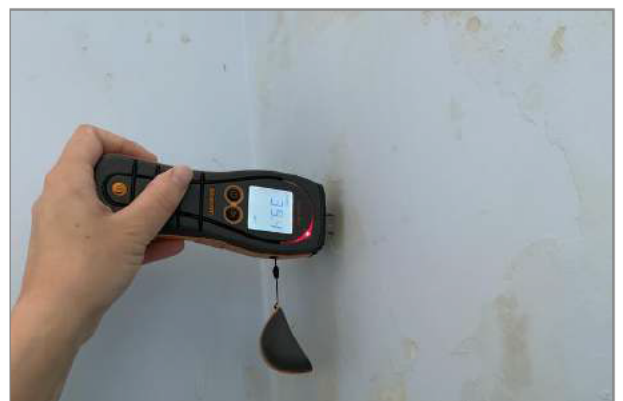
Photo - 61 Damp found to staining to first floor bedroom wall
