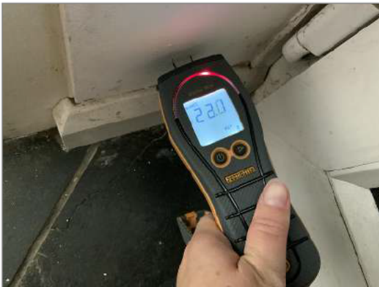
Photo - 52 Damp to left of lower ground floor door
