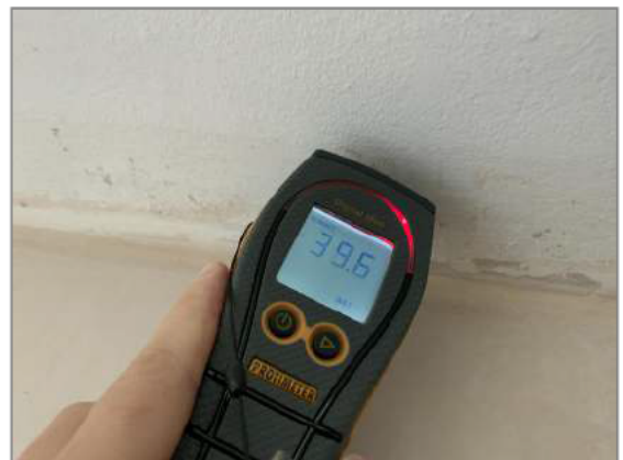
Photo - 46 Damp found to ceiling above second floor chimney breast
