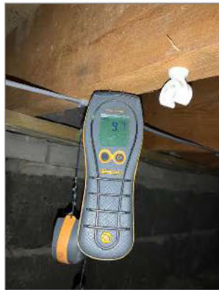
Photo - 88 Damp meter reading under kitchen
